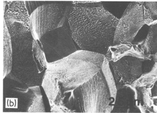
Figure 4 Fracture surfaces of tensile specimens taken from stress relieved flanges and strained to fracture at room temperature. (a) Cast No. 1, transgranular ductile fracture. (b) Cast No. 2, intergranular fracture.
