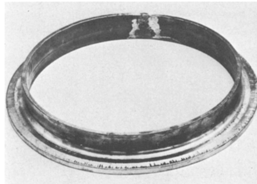
Figure 1 A pipe flange of aluminium brass made by welding together the two ends of an extruded "L" profile.
